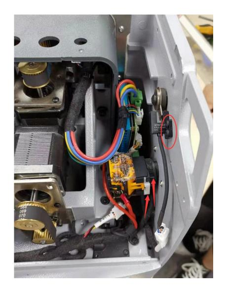
Take out the 2 screws in the sensor of protective shell and pull the white buckle to disconnect the switch button then loose the right buckle for take out the switch button, the red arrow is point to the buckles of switch button
