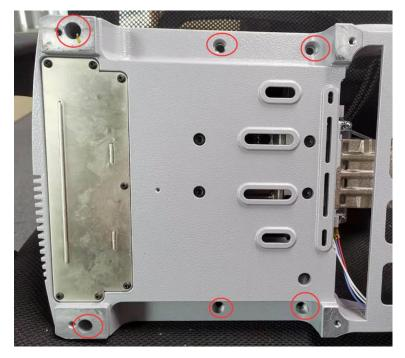
Turn over the machine like picture show and remove the foot base and 6 screws
