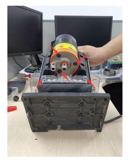
Take out the whole motor part and take out the screws like picture show for remove the led bar and mounting plate of probe
