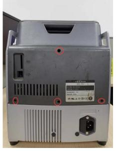
Take all screws like picture show ,and remove the protective shell , screen module , side accessories
