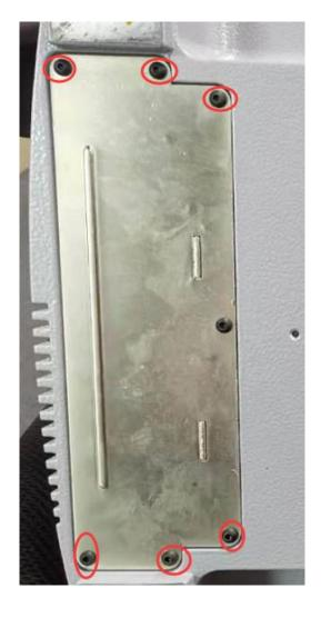
Take out all screws for remove the cable fixture and cables and start to fix all cables back
