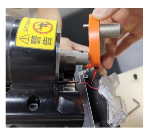
Take out the screw of the cable M-D-P and cut the cable like right picture show, then pull the led bar for take out the whole cable
