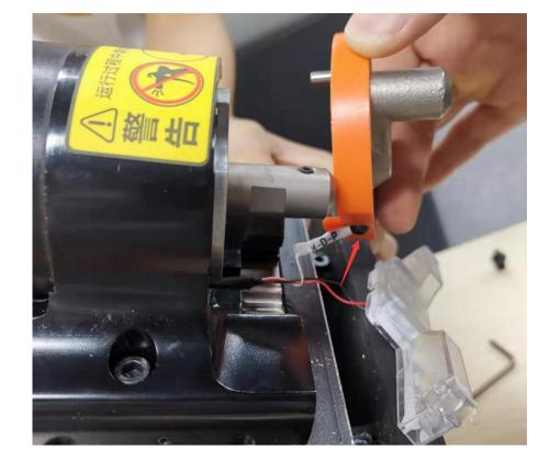
Fix the M-D-P cable after insert the whole cable and fix back the mounting plate of probe and led bar ,first fix back the plate then fix the led bar , then white part mark with 'M-D-P' should be in the hole and can not twist or bend it , you can pull the cable in another side for fix that
