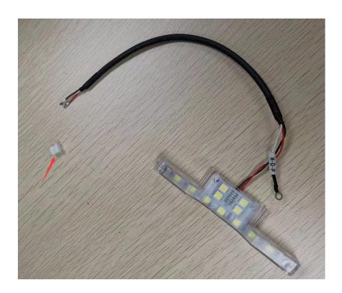
Take the led bad and cable what I send you like the left picture and insert the cable in that hole and through it to another side
