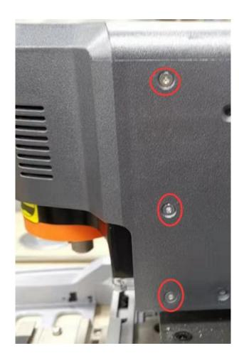
Take out those 6 screws for remove the shell of main motor
